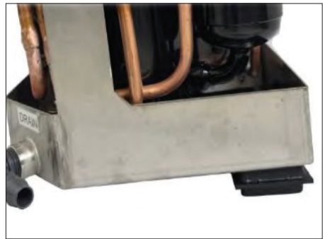
In the above picture, shims have been used to improve the condensate drainage.
