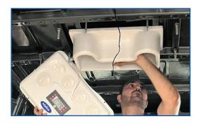
9. After having the Styrofoam already molded, go back to the roof and peel the sticker from the foam gasket gradually while sticking it on the mounting plate, making sure its outside the 4 screws to prevent water leaks. Manually shape it to a square shape while positioning.
