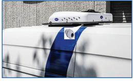
12. From inside the vehicle, you will have the unit upside down and ready to tighten the Fixing screws on the nuts using the locating plates provided.
