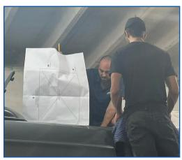
Drill the 4 holes for the pass-thru bolts. (For easier fit, use a unibit drill to oversize the holes)
