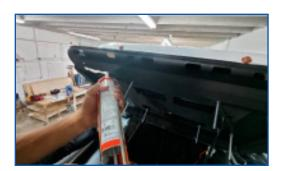
8. Once the unit is sitting on top of the roof, take the wire harness and drill a hole in the selected location to pass it thru the roof, using a Cable Gland, well sealed with the same sealant used for the gasket to prevent water leaks.
