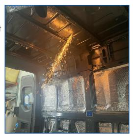
3. Once the opening is cut you must smooth the edges and paint it with anti-rust paint.
