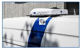
9. From inside the vehicle, you will have the unit upside down and ready to tighten the mounting screws on the nuts using the L bracket positioning plates provided. If necessary, adjust the plates to distribute the stress on the roof surface.
