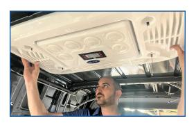
11. Finish the installation by plugging the Led Lights and clip it on its location to cover the nuts.
