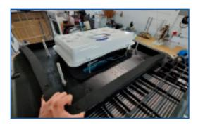
Once the gasket is positioned, we recommend using a UV rated sealant before lifting, orient the unit facing the roof of the vehicle.
